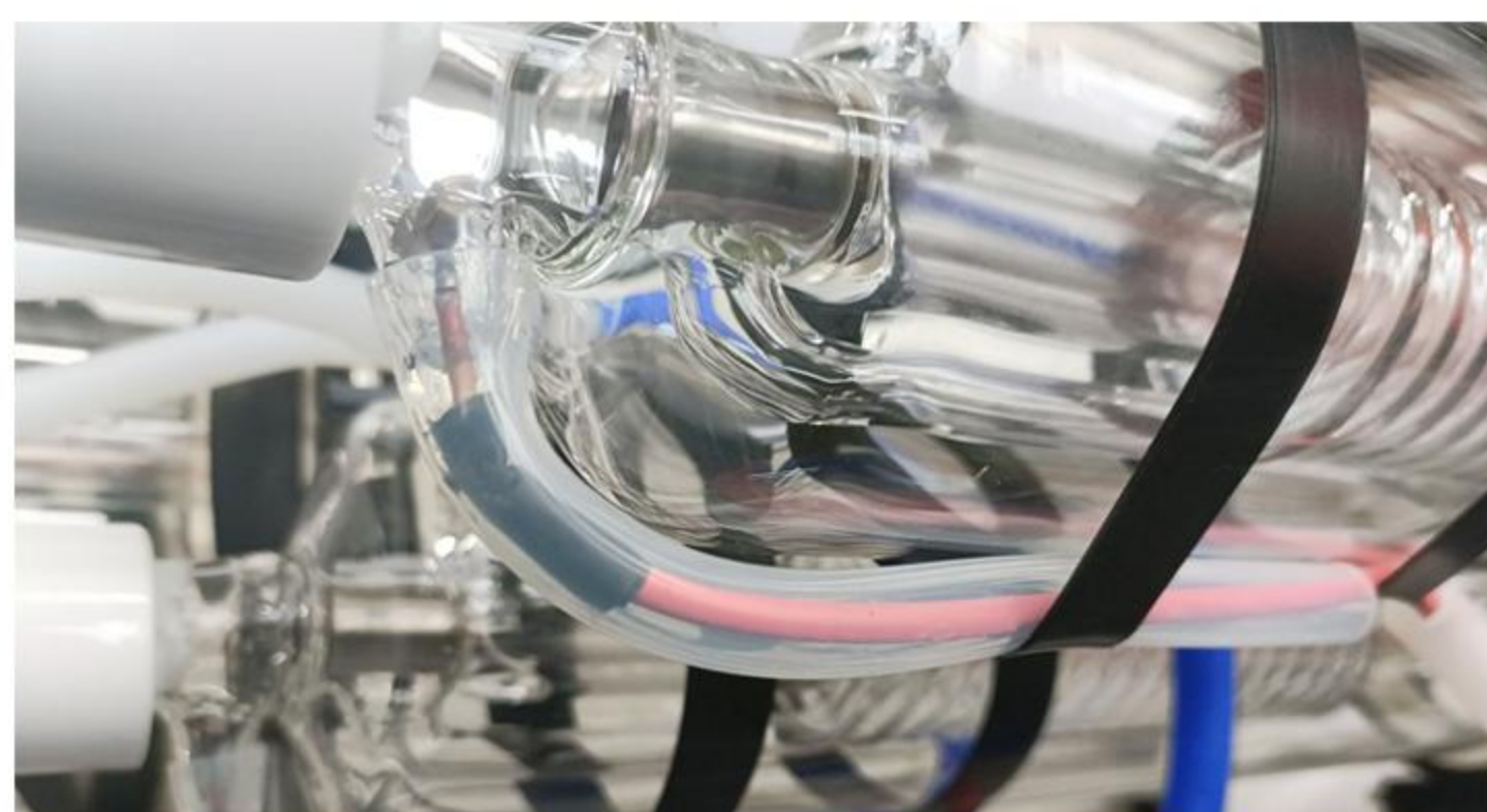
High-Voltage Wire Insulation
